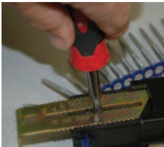
Remove screw using Phillips screwdriver. Align marks on nosepiece with locking boss for proper fastener lengths. To tighten screw, depress the nosepiece using slight pressure. Tighten the screw to make sure it is snug against the slide-body.
