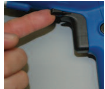
Be sure screw gun is operating in forward (clockwise) direction. Screw will not advance and bit will be damaged otherwise.
