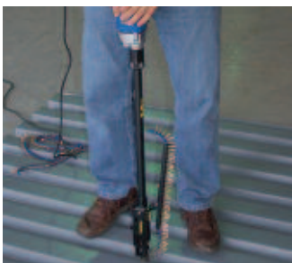
Pull the trigger to start the motor, press the nosepiece with constant force against the work surface. Do not remove the tool from the work until the clutch disengages and the bit stops rotating, signaling a fully driven screw. The next screw will be automatically fed into place when the tool is removed from the work. This tool has a depth-sensing clutch and will automatically disengage making a click ratcheting noise signaling a completed drive.
