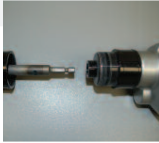
Insert inner rod into center of adapter and screw gun. Push down until rod clicks into place. Slide outer extension pole over inner rod and thread onto screw gun adapter.
