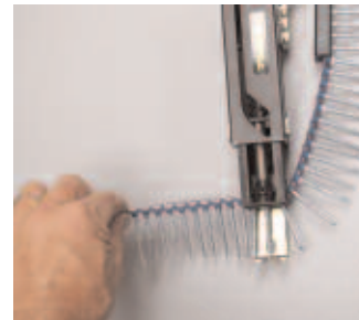
To remove the strip, pull it through from the bottom of the nosepiece.
