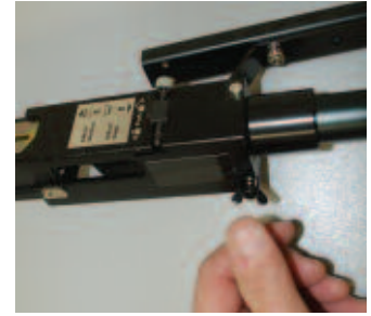
Install the screw attachment making sure it is positively seated. Tighten wing nut until snug.
